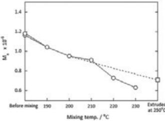
Figure 3. The change in the molecular weight of the blends with mixing temperature setting the mill gap at 0.1 mm.
