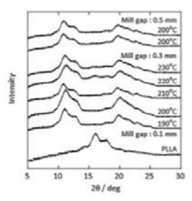
Figure 6. WAXD spectra of the blends prepared at various temperatures setting a mill gap at 0.1 mm. Data for the pure PLLA and the blends pre- pared at 2008C setting mill gaps at 0.3 and 0.5 mm are added for comparison.
