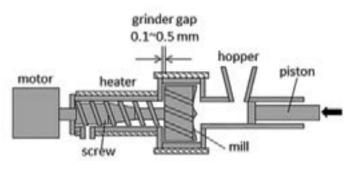
Figure 1. Photograph and a schematic diagram of the mill-type melt- mixer used in this study.
